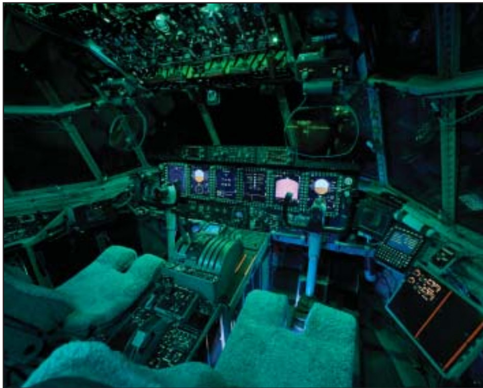
A photo of the C-130 avionics modernization program modified flight deck. Six digital displays and the flight management system Boeing developed for its newest
