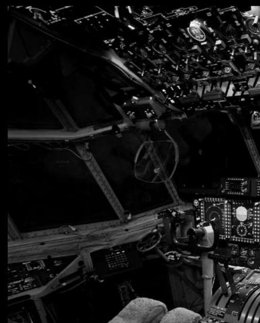
The cockpit of the AMP upgraded C-130, above, C-130s. The analog instrumentation familiar to pilots is gone, replaced by six liquid crystal flat screen monitors under two plastic "heads up" displays that allow pilots to get the information they need while maintaining their focus outside the cockpit.
