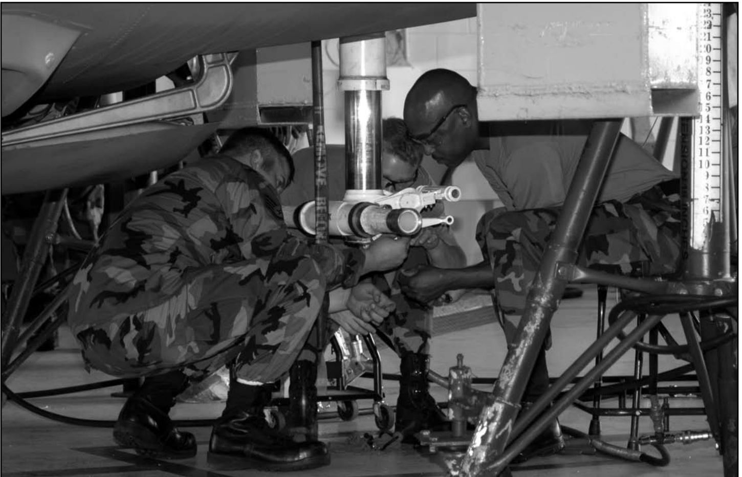
From left, Staff Sgt. Jason French, Senior Airman Robert Bing and Staff Sgt Joseph Stone install a nose landing gear tow fitting. The fitting is used for handling the aircraft on the ground.
