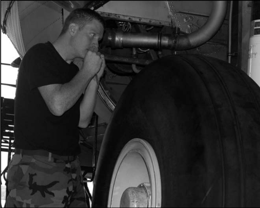
Senior Airman Shane Prater prepares to install a safety chain in the main landing gear wheel well as part of aircraft 9101's isochronal inspection.
