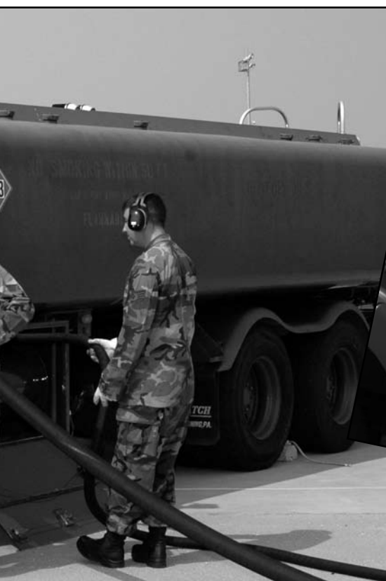
Staff Sgt. Andy Hernly pulls the 2.5-inch hose from an R-11 refueler in preparation for a refueling operation.
