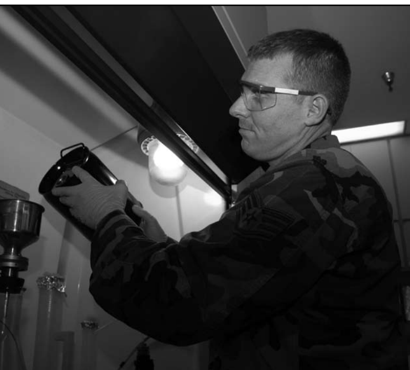
Staff Sgt. Ronnie Warner conducts a bottle method test to determine if a sample of JP-8 meets strict Air Force specifications for quality. This test is performed each time jet fuel is received at Maxwell. The test is also performed randomly at 90-day intervals and sent to the area laboratory at Wright Patterson AFB, Ohio, for comparison analysis.
