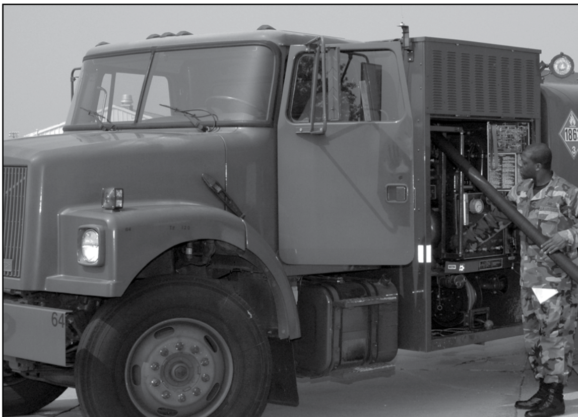
Fuel flight members conduct a vehicle checkpoint operation on a R-11 refueling vehicle before it's sent to the flightline to service aircraft. The R-11 is capable of issuing jet fuel such as JP-8 at 600 gallons per minute.
